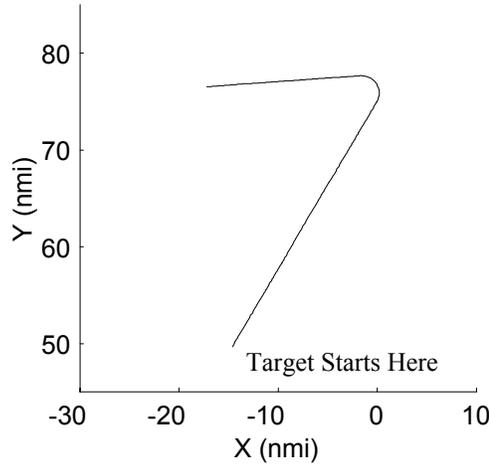
Figure 12: Target trajectory 2: 500 *kn* target making a 3g turn.
