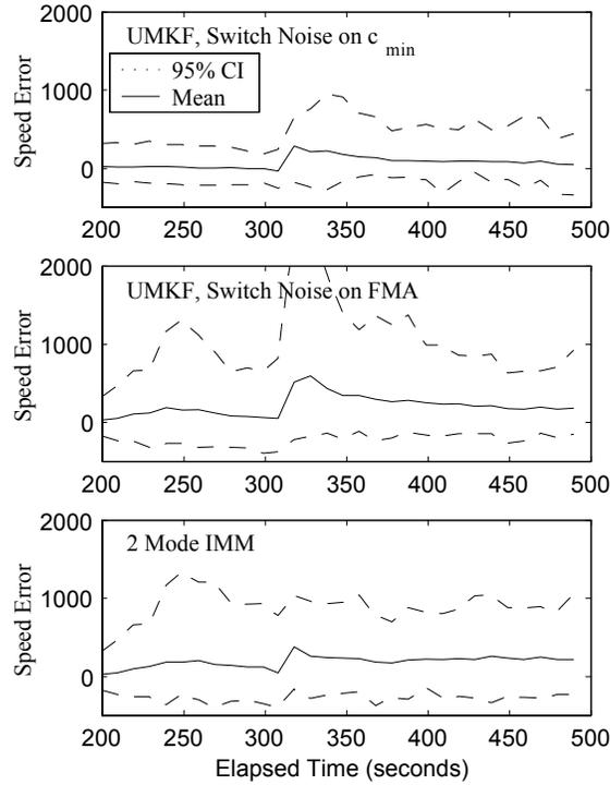
Figure 11: Mean and 95% confidence bounds of position error for the target in test case 1. From top to bottom (i) mode switching tracker using  $c_{\min}$ ; (ii) mode switching tracker using innovation FMA; (iii) 2 mode IMM tracker.
