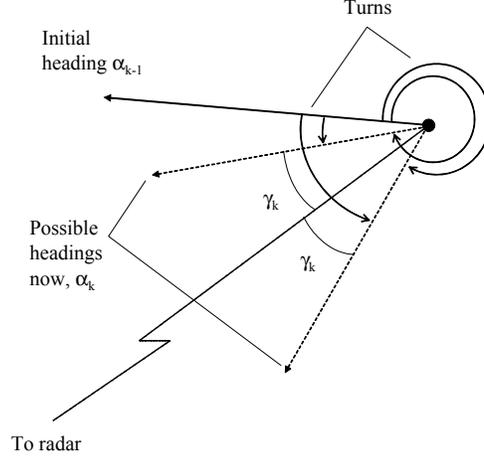
Figure 2: Four possible turns, two to the left and two to the right, such that the actual and measured range rates are equal.
