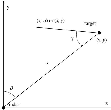
Figure 1: Problem space: Cartesian frame with radar fixed at the origin and a moving target.
