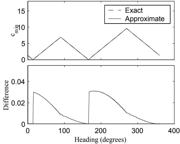
Figure 4:  $c_{\min}$  computed using the exact and approximate method (top), and their absolute differences (bottom) for a 400 *kn* target at 150 *nmi*.
