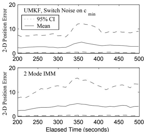
Figure 13: Mean and 95% confidence bounds of position error for the target in test case 2. From top to bottom (i) mode switching tracker using  $c_{\min}$ ; (ii) 2 mode IMM tracker.
