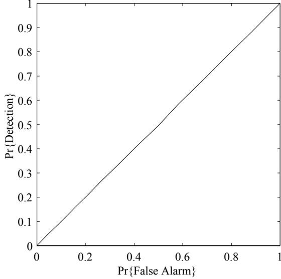
Figure 8: ROC for a threshold test of a fading memory average of position residuals.
