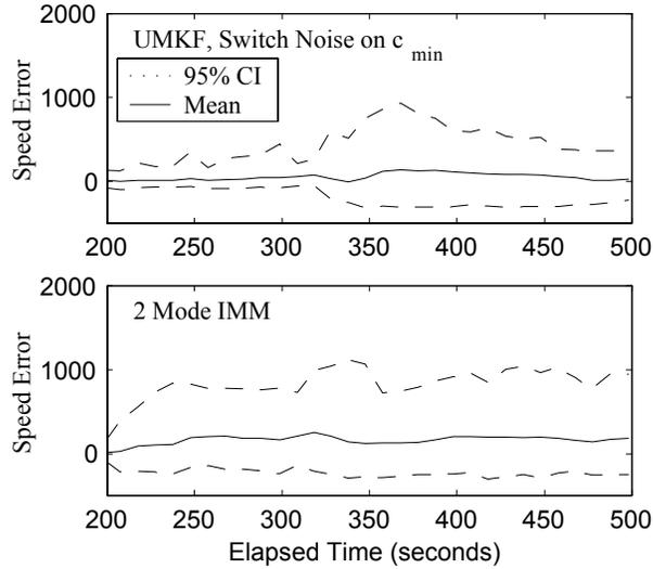
Figure 14: Mean and 95% confidence bounds of speed error for the target in test case 2. From top to bottom (i) mode switching tracker using  $c_{\min}$ ; (ii) 2 mode IMM tracker.
