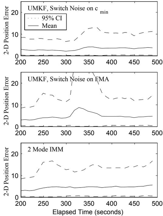
Figure 10: Mean and 95% confidence bounds of position error for the target in test case 1. From top to bottom (i) mode switching tracker using  $c_{\min}$ ; (ii) mode switching tracker using innovation FMA; (iii) 2 mode IMM tracker.
