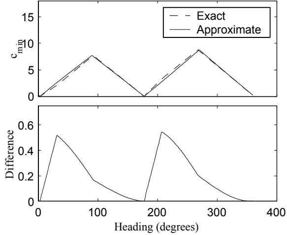
Figure 3:  $c_{\min}$  computed using the exact and approximate method (top), and their absolute differences (bottom) for a  $1000kn$  target at  $50nmi$ .
